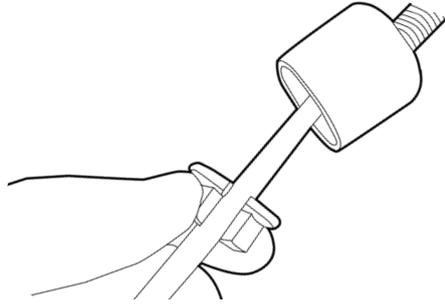
3. Discard the cap by cutting through it safely with a side cutter.
