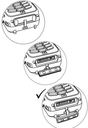
2. Press down the latch button and then gently rotate it up to open the latch. Place the Iridium Extreme handset into the PotsDOCK Extreme.
