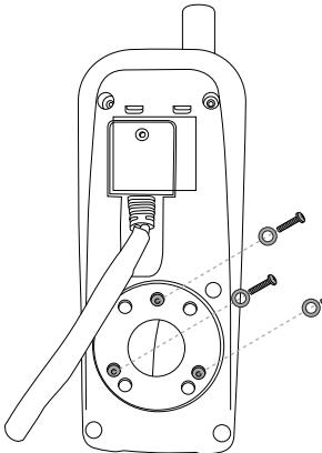
2. Secure the second pivot base to the location you have selected for mounting the PotsDOCK Extreme. (Screws not supplied)
