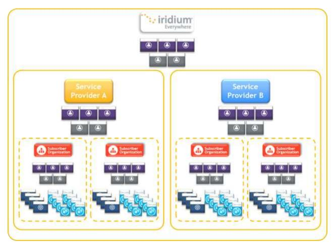
There are three levels of hierarchy within the Iridium PTT Command Center: the Iridium level, the Service Provider level and the Subscriber Organization level. The figure below illustrates this relationship.
